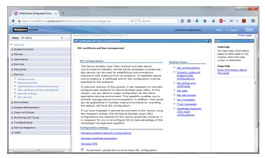
1. On the left pane, expand 'Security' and click 'SSL certificate and key management'. Under 'Configuration settings', click 'Manage endpoint security configurations'.
