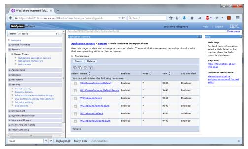
3. Against their respective names, the secured connection is available under the column 'SSL Enabled'. Click 'WCInboundDefaultSecure'.
