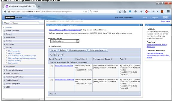
This screen is used for attaching the key store to the application server.
