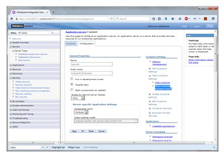
2. Go to Configuration tab and click 'Web container transport chains' under 'Container settings'.
