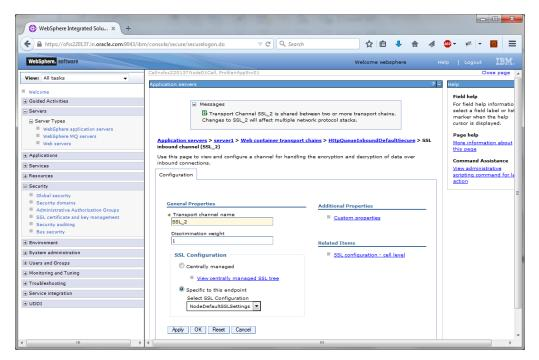
Select the configured SSL from the list of SSL configurations. Click 'Apply' and save the changes.
